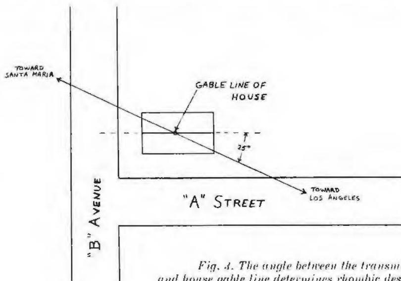
Fig. 3. The angle between the transmitter and house gable line determines rhombic design.
