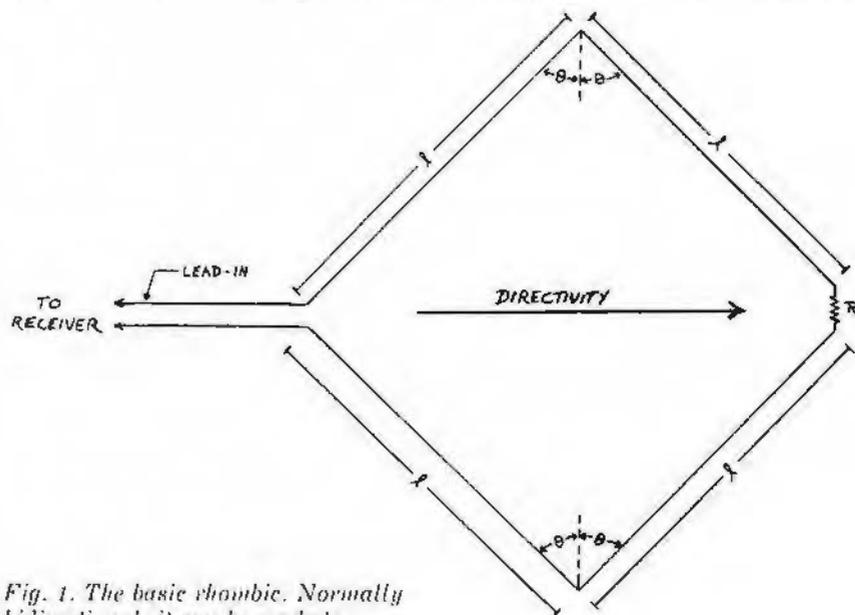
*Fig. 1. The basic rhombic. Normally bidirectional, it can be made to focus in one direction by adding the resistive termination.*
